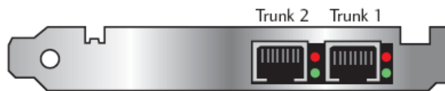
Figure 5-4: Trunk Status LED Locations
